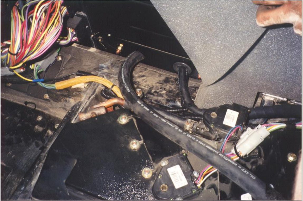
Hoses passing through hose plate (supplied) at rear of cab.
